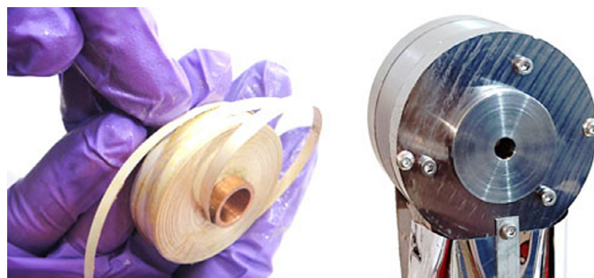
Figure 14. A 2T shielded dual pancake coil HTS magnet with a soft iron aperture insert.
